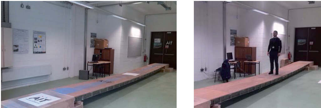
Figure 1. (a) Completed Laboratory Scale FRP Composite Footbridge (b) with person at midspan
