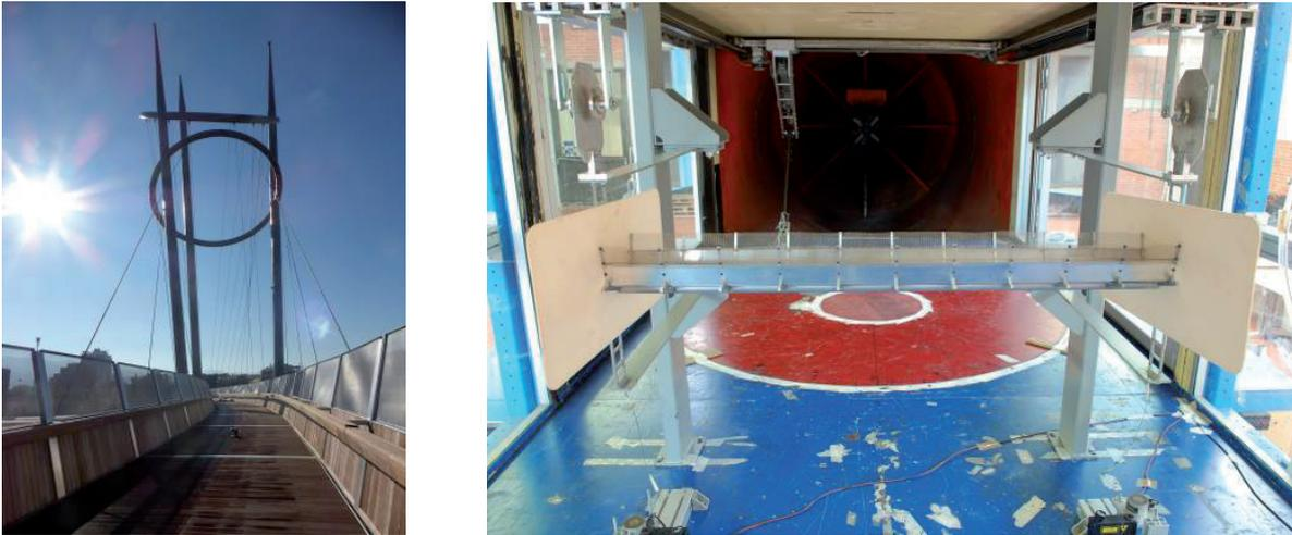
Fig. 1. View of the footbridge (left - Terni, Italy); sectional model in the wind tunnel (right - CRIACIV lab.).
