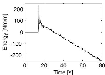
Fig. 3: Example of Total Mechanical Energy of Damper Actuators
