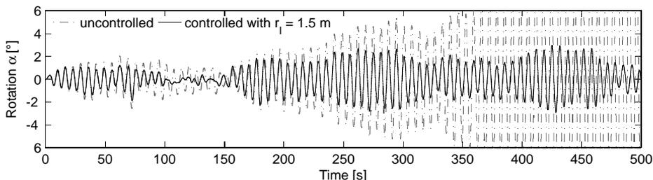
Fig. 2: Numerical Simulations in Time Domain: Controlled and Uncontrolled Response for Mean Wind Speed of 39.7 m/s and Rotor Length of 1.5 m
