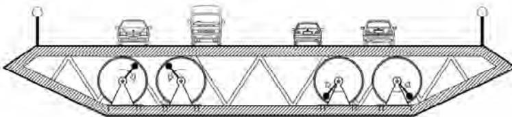
Fig. 1: Proposed Damper Configuration
