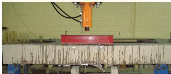
Fig. 2: Crack pattern, obtained by FE simulation and the crack pattern observed in the test
