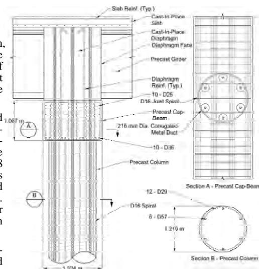
Figure 1: Details of the full scale connection
