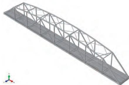
Fig. 2 FE model of the experiment bridge.
