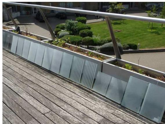
*Figure 1. Various cast glass samples from various manufacturers’ world-wide. Line up on Architect’s terrace. Photo by author.*
