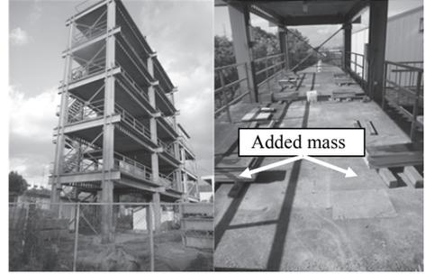
Fig. 1: The target structure with mass
