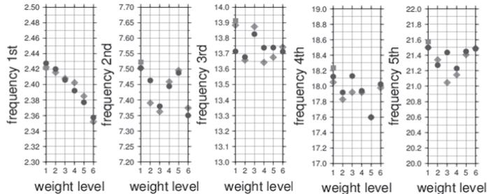
Fig. 2: Comparison between observation (●) and theory (◆) for natural frequencies of five modes with known mass loading on the weight
