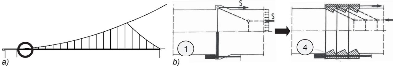
Fig. 1 a) Suspension bridge with the anchorage of the main steel cable on the deck b) ① → ④ train of thought behind the saw-tooth connector [1]
