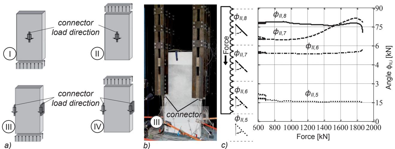
Fig. 2 a) Four different types of specimens b) compression test with the connector on the edge of the slab c) angles of struts (Strain Gauges)
