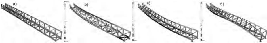
Fig. 2: FEM model made due to design documentation and geometric forms of natural frequencies for whole footbridge
