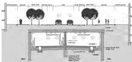
Traffic flow requirements imposed 2 lanes in the southbound and 3 lanes in the northbound direction. The tunnel section has a clear height of 4.80 m and depending on the number of lanes a clear width of 6.00 m to 11.75 m respectively. In the areas of on- or off-ramps, the tunnel section is widened to accommodate additional lanes.
