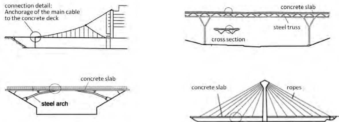
Fig. 1: Examples for the application of saw tooth connectors in bridge design
