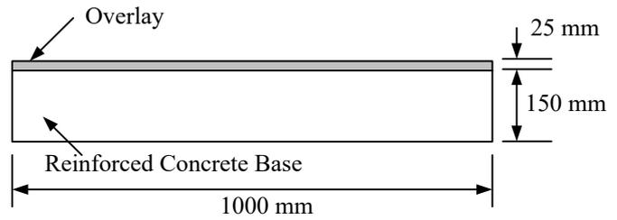
Fig. 1: Overlay Specimen Details
