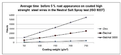
Fig. 1. Corrosion performance of Zinc, Bezinal and Bezinal 3000 in the Neutral Salt Spray test.
