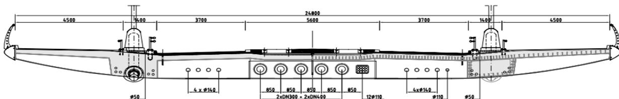
*Fig. 2: Structural cross section of the bridge*
