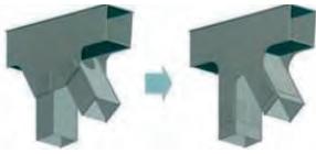
Fig. 2: All welded compact truss panel point in comparison with conventional one
