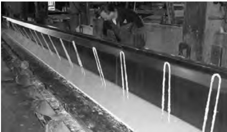
Fig. 3: Installing the top part of the mold
