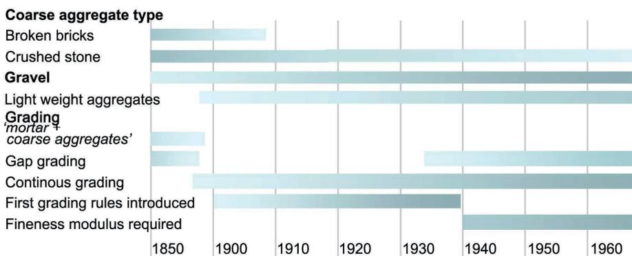
Figure 2. Timeline indicating possible types of coarse aggregates and concepts of grading binders applied for historic (reinforced) concrete in the Netherlands.
