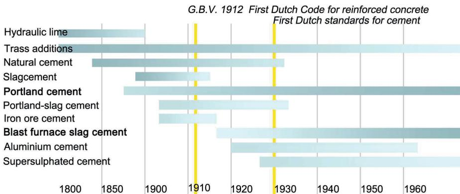
Figure 1. Timeline indicating possible binders used for historic (reinforced) concrete in the Netherlands. G.B.V. stands for Gewapend Beton Voorschriften, Netherlands Code of Practice for reinforced concrete.
