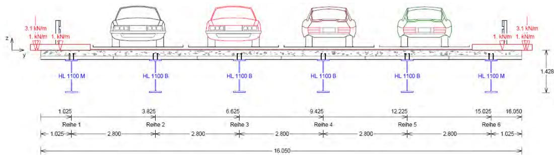
Fig. 1: Cross section RQ15,5 from [6]
