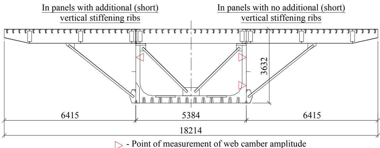
*Fig. 1: Cross-section of the superstructure and points of the camber amplitudes measurements*
