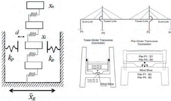
Fig.2. Schematic figure of pounding model at tower-girder and pier-girder connections
