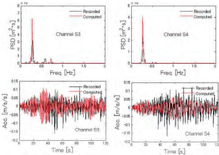
Fig.3. Comparisons between model and measured acceleration responses and spectra for two locations on the wind shoes on P2 (S3) and P3(S4)
