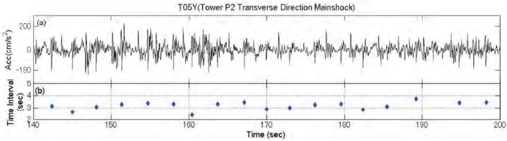
Fig.1. Close-up look at the tower transverse (in-plane) acceleration at the tower-to-girder connections shows (a) periodic impulse response for and (b) Time interval between consecutive impulses during
