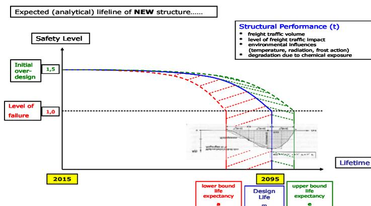
The starting point of the bridge's service life – in terms of the safety level – is according to the initial overdesign and depends on the applied design code and certain safety consideration in the course of the static calculations.
