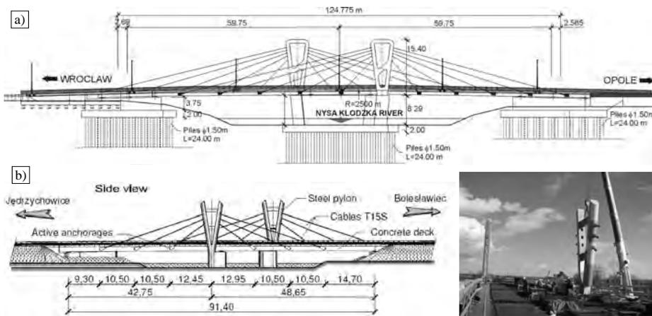
Fig. 2: a) Side view of bridge in Skorogoszcz, b) side view and pylon erection of viaduct in Wykroty
