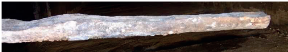
Figure 2. Corroded reinforcement bar.
