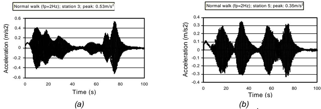
**Fig. 2 Walking of single pedestrian at a pacing rate of 2Hz: (a) 1/3<sup>rd</sup> span; (b) Mid-span**
