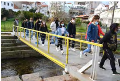
Fig. 5. Crossing footbridge by 18 pedestrians during ambient vibration test. General view and time records
