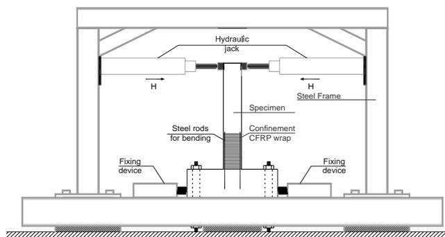
Fig. 2: Testing Stand Set-up
