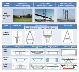
Figure 1. Load Bearing Elements of CSB & EDB
