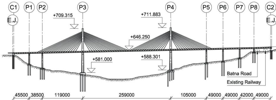
*Fig.1: General arrangement of Main Bridge, elevation*
