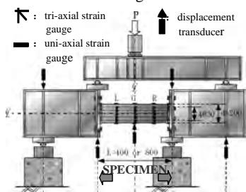
Fig. 1: Test Setup and Measurement Devices
