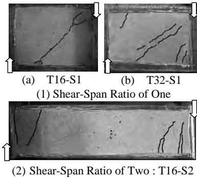
Fig. 2: Cracks in Core Concrete
