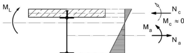
*Fig. 1: Structural behaviour of a normal height composite girder*
