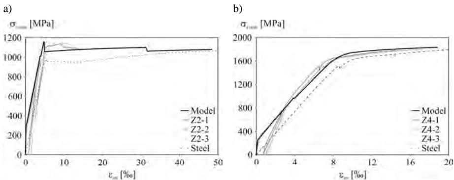
Fig. 1: Stress-strain-diagrams of reinforced UHPFRC tension chords: a) Specimen Z2, b) Z4
