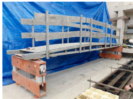
Fig. 1. (left) Bending-active UHPFRC bow-string prototype, and (right) bending-active UHPFRC lenticular beam prototype
