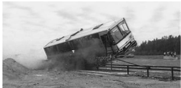
*Figure 1: On left, impact of car weighing 937 kg against Finnra H2 vehicle parapet with 2-pipe rail at 104 km/h impact speed and 20° angle. On right, impact of bus weighing 13.12 tons at 81 km/h impact speed and 19.1° angle. (Courtesy of Helsinki University of Technology)*
