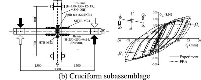
Fig. 5: Load-Deformation Relationships (Beam-to-Minor-Axis Column Connection)
