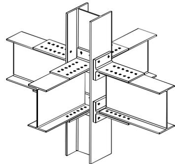
Fig. 1: Unstiffened double split-tee beam-to-column bolted connection
