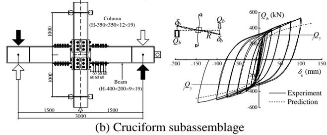
Fig. 3: Load-Deformation Relationships (Beam-to-Major-Axis Column Connection)
