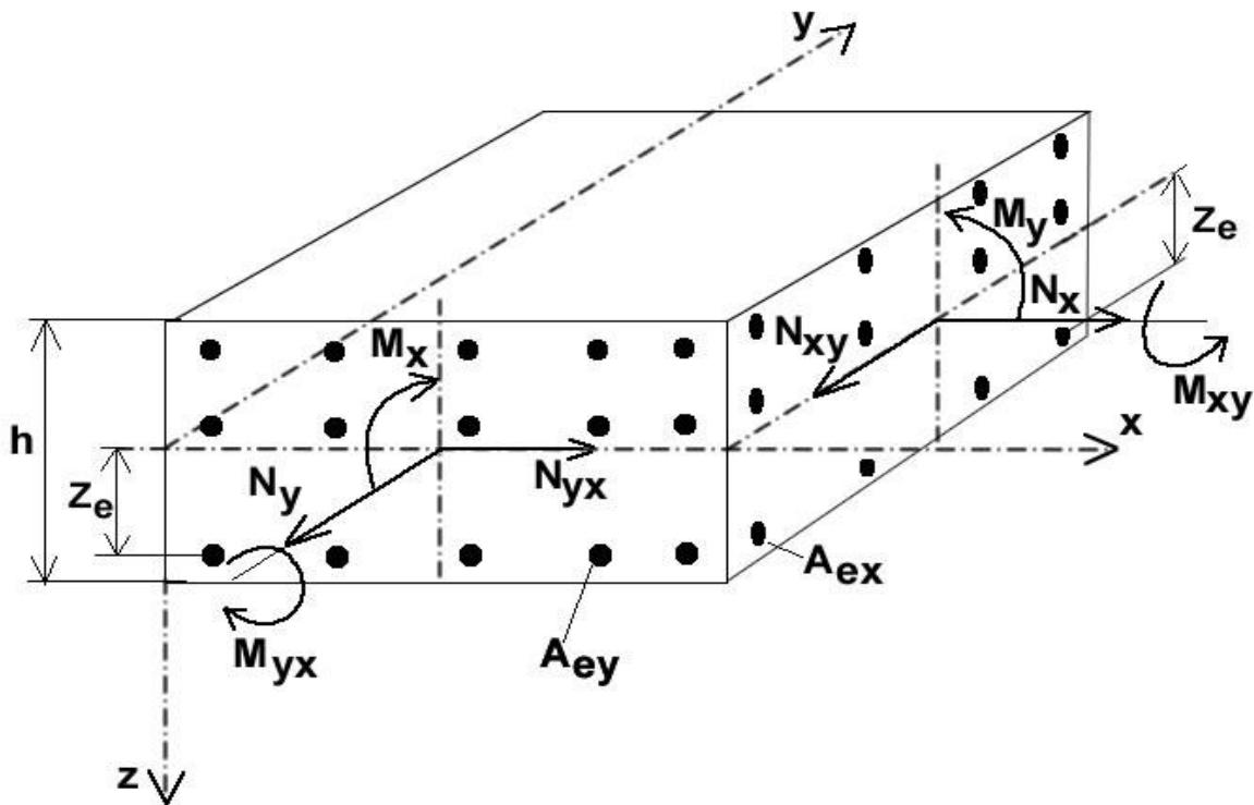
Fig. 1: Slab Element
